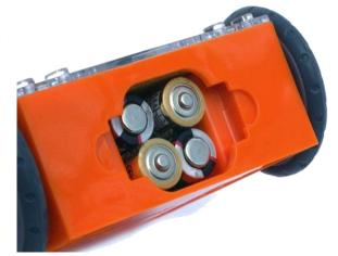
Ensure the batteries are in the right way.
