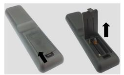
• When loading the battery, check if the polarity of the batteries is correct.
